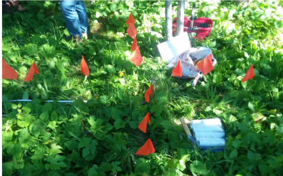
Figure 2: Soil sample collection layout. Orange flags mark 25, 50, 75 and 100 centimeters from the base of the plant in four cardinal directions, and soil samples were taken from each flagged site.
